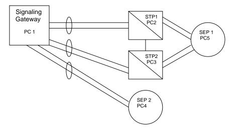
Figure 6 demonstrates a Signaling Gateway routing to two SS7 Signaling End Points (SEP). The first SEP is reached by a pair of STPs, while the second SEP is reached directly from the Signaling Gateway. Example MML for the above configuration is:
